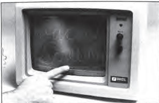
Series 3000 Touch Screen  $\frac{1}{2}$ " electrode system permits concealment under bezels of IBM 5153, 5154, 5151, Princeton Graphics HX-12 monitors. Integration includes serial controller, power supply, cable, documentation; \$895 in quantities of 100. **Interaction Systems, Inc., 24 Munroe St., Newtonville, MA 02160; 617-964-5300; TLX 753582.**
