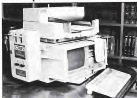
The IBM/MS-DOS compatible CD *InfoMachines* are computer systems installed with software providing capabilities from data entry to printing. When the correct change is deposited, the unit powers up for patron use. Model 2000, which includes a high-speed 80286-chip-based processor unit with monitor, a laser printer, and access control capability, sells for \$7,999. Model 1000 with IBM-XT
